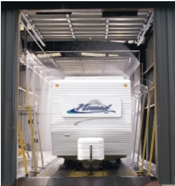
All Nomad units are tested for 15 minutes in a high-pressure shower spray to guarantee that they are watertight.
