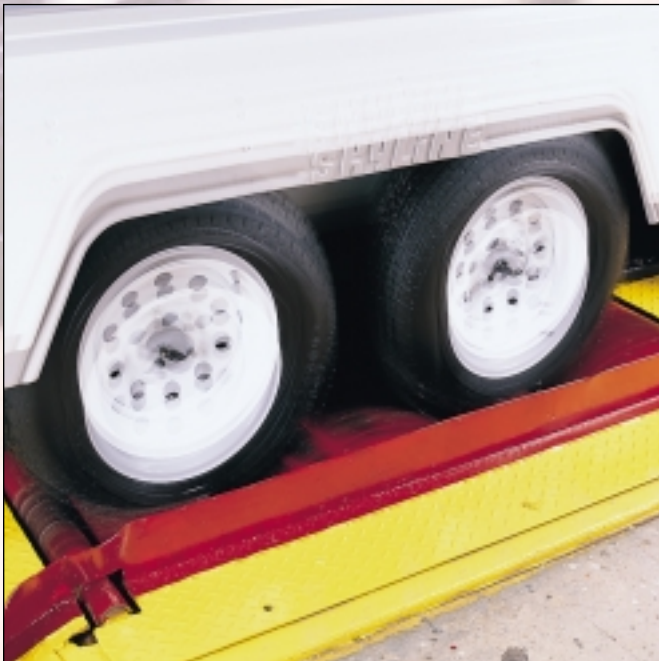
A shake-simulator test is performed for 10 minutes to detect any problems before leaving the factory.
